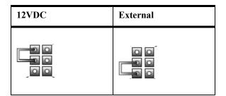
**Note:** The power source selected by the jumper settings shown above configure the power source for the relay. It does not configure the power source for the panel.
